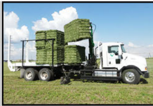
2. The arm raises, swivels and lowers the bale onto the bed. Once two bales (three 3X3s) are loaded, they sweep back.
