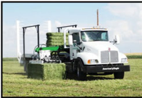
1. The robotic arm lowers to the side and sinks its 16 tines into the bale.
