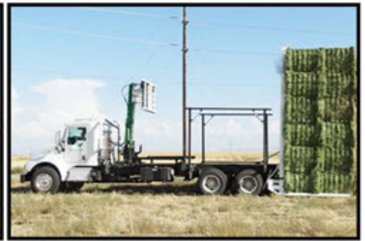
3. When full, the bed can be tilted past 90 degrees to stack up to 6 high. Stacks are tight and onisistent.
