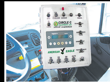
Programmable controller is sealed from dust or moisture. Only 7 limit switches for fully automatic operation.
