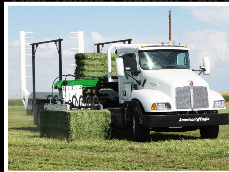
1. The robotic arm lowers to the side and sinks its 16 tines into the bale.
