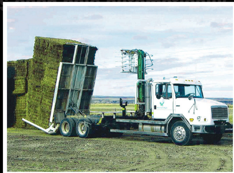
3. When full, the bed can be tilted past 90 degrees to stack up to six high. Stacks are tight and consistent.
