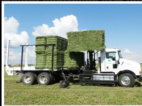
2. The arm raises, swivels and lowers the bale onto the bed. Once two bales (three 3x3s) are loaded, they are swept back.
