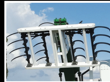
The "Sure Grip" big bale claw tightly grasps even loose and tattered bales. The 8 foot, 2-ton capacity robotic arm is equipped with a mechanical deceleration valve.
