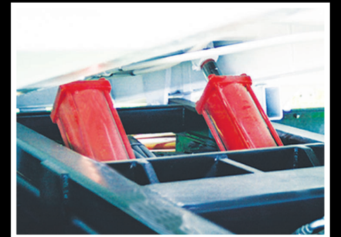
Dual 3000 psi bed lift cylinders with double-acting safety valves ensure that the load will be lifted safely, smoothly, and quickly.
