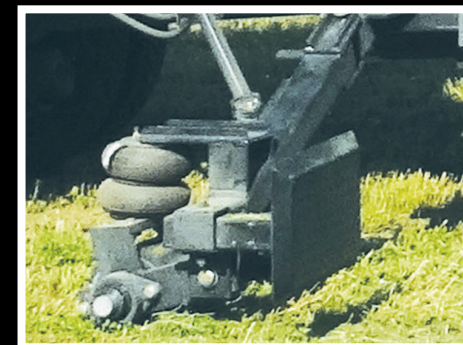
Retractable bale catcher arm with "air-ride" suspension provides stability while picking up bales.
