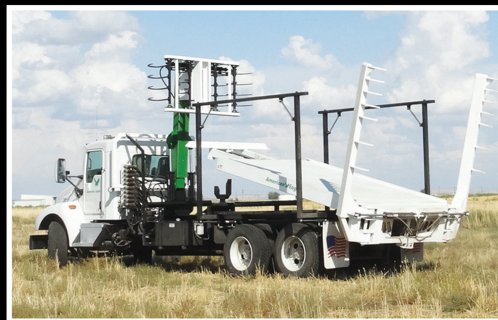
Retractable bale catcher arm with "air-ride" suspension provides stability while picking up bales.
